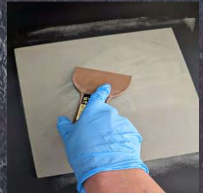
Use the rubber spatula for making patterns. Move it left and right alternately
