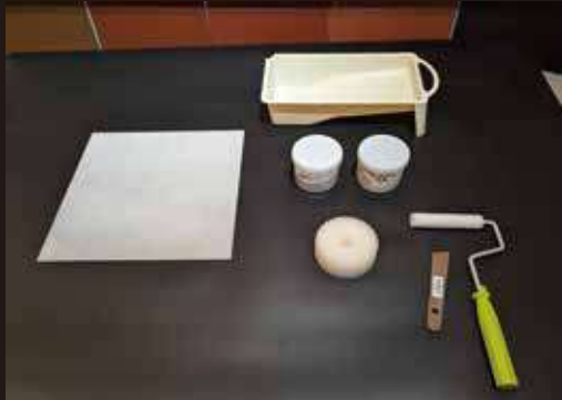
Cement panels, coating materials, rollers, sponge
