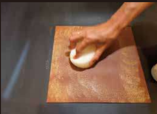
Apply in pats. Apply a thin layer. .Applying too much will spoil the aesthetic appearance.
